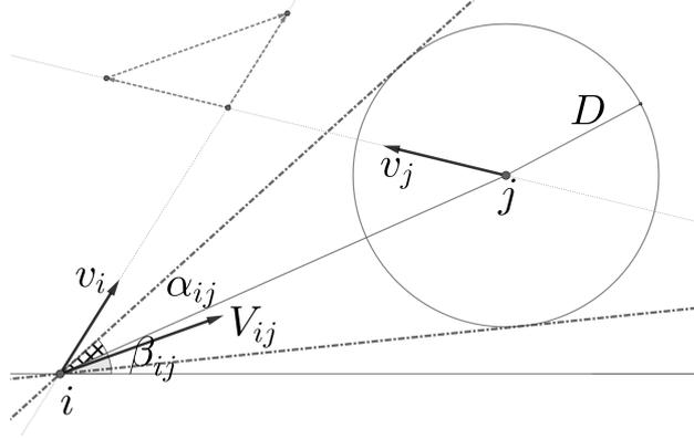
FIG. 1: Geometric analysis of conflict between two aircraft based on relative velocity
